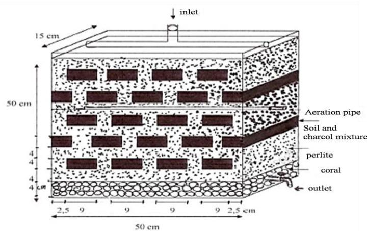
**Figure 2: Design of MSL system**
