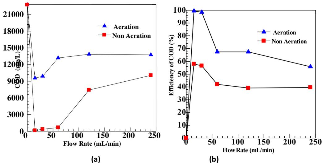
Figure 6. Effect flow rate of tofu industry wastewater on (a) COD concentration and (b) removal efficiency of COD
